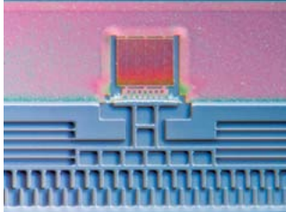
MEMS red pitch variable guided-mode resonant grating (1000x)
