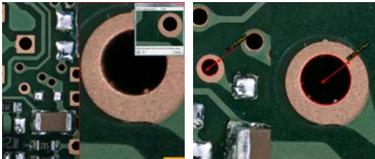
Each display area can be moved independently on the split screen. Images of different magnifications can be measured individually.
