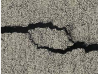
Cracks in stainless steel (300x)
