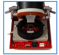
DUT Interfacing: Test Socket Alignment - latches and guide pins provide easy and secure connections to the test socket. Soldered Component Alignment customized interfaces to accommodate PCB layout and chip geometry.
