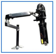
**Bench Stand**: Free-motion stand and boom provide manually positioning of the Thermal Head over the DUT. (P/N SA214360)
